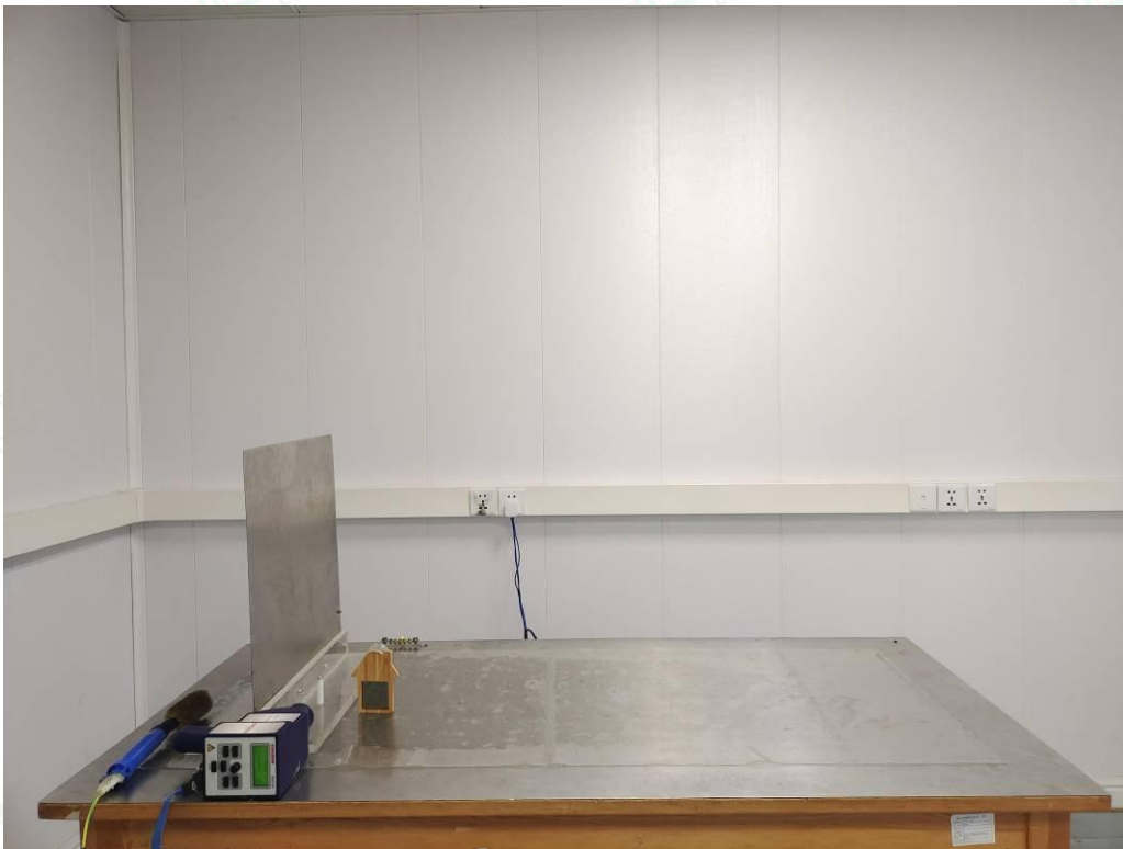
Test Setup Photo of Electrostatic Discharge Test
